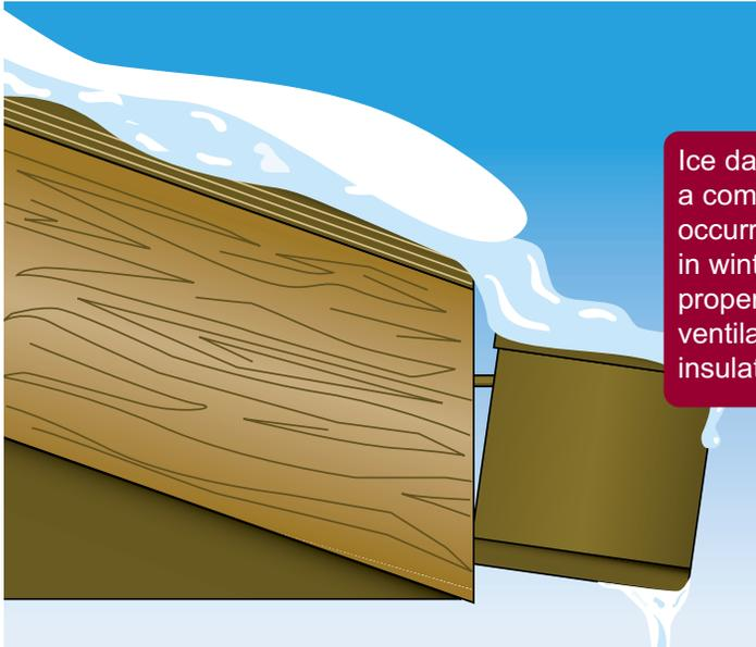
Ice dams are a common occurrence in winter without proper attic ventilation and insulation.
